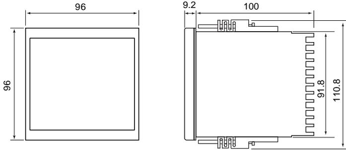
For mounting of the controllers, panel thickness must be between 1 to 10mm. When mounting multiple controllers close together, the panel strength should be checked to ensure proper support.
